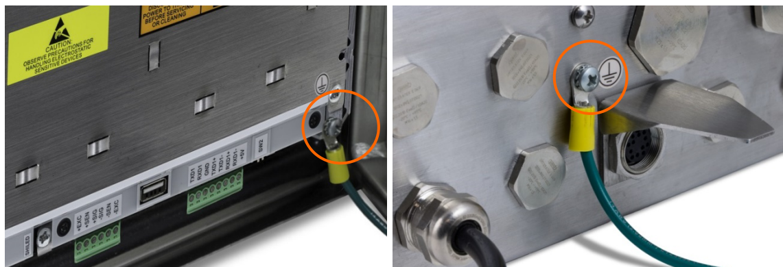
Figure 2-5: Grounding Points, Panel-mount (left) and Harsh Enclosure (right)
