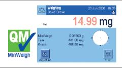
MinWeigh warns you when your sample weight is below the defined minimum weight. Small minimum weights increase the yield of the substance and are therefore cost-saving. Our recommendation for typical minimum weights: from 0.6 mg: UMX2
