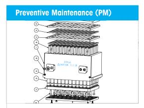
Preventive maintenance is essential to maintaining peak performance. Rainin's comprehensive preventive maintenance includes cleaning and re-greasing pistons and replacing nozzle O-rings. We strongly recommend a warranty upgrade as it includes one preventive maintenance (PM) event during the manufacturer warranty period.
