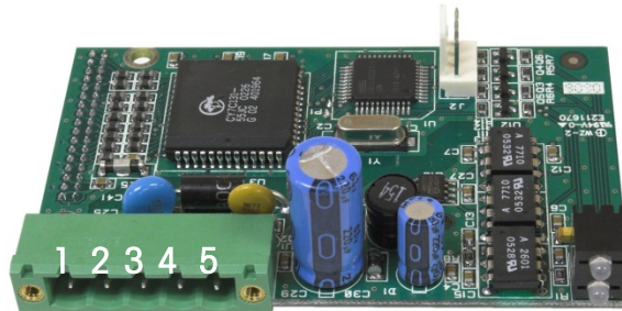
Figure 2-103: DeviceNet Option Board Connector Pin Numbering
