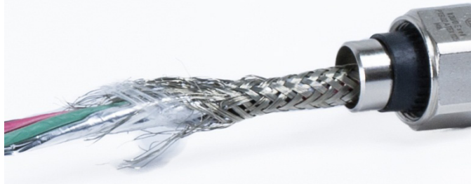
Figure 2-59: Inner Sheath Frayed
