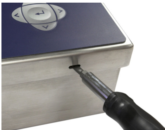
Figure 2-4: Opening the Harsh Enclosure, Alternative Method
