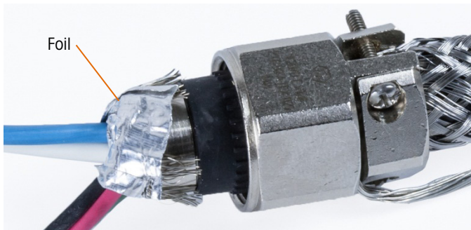
Figure 2-62: Foil Cut Back and Folded Over Ferrule
