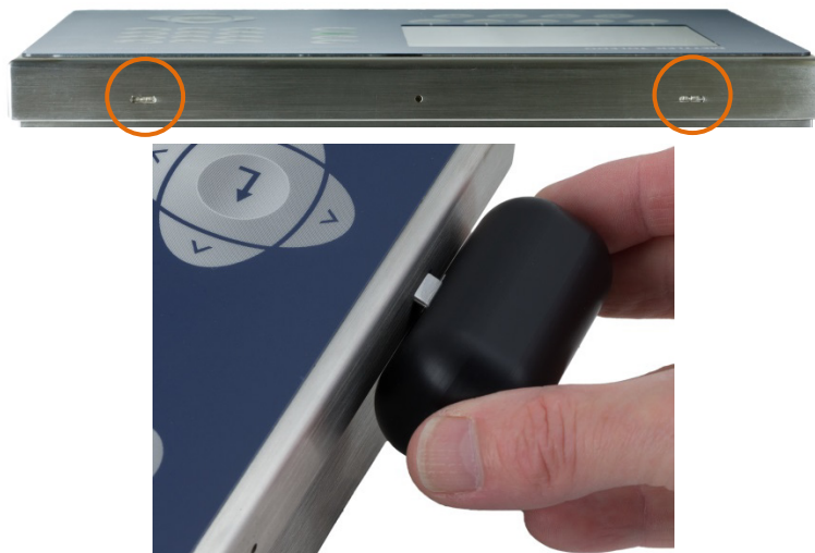
Figure 2-2: Opening the Harsh Enclosure, Preferred Method
